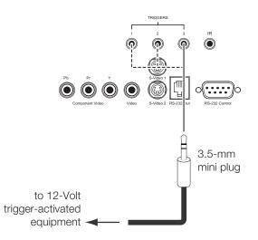
Figure 3-10. Connecting 12-Volt Trigger Outputs
